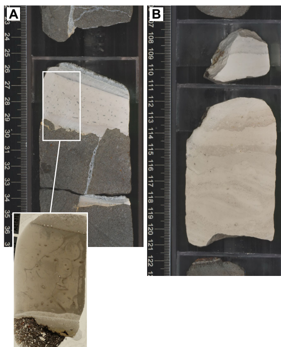
Figure F15. Sedimentary infills and intervals in the volcanic basement, Hole U1575A. A. Yellow-white burrowed nanofossil limestone (Lithofacies 1; 24R-1, 22–37 cm). B. Yellow-white burrowed nanofossil limestone with foraminifera (Lithofacies 2; 39R-3, 106–123 cm).
