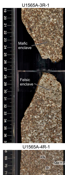
Figure F6. Unit II macroscopic observations, Hole U1565A. Top: presence of centimeter-scale enclave is highlighted. Bottom: dominant mineralogy is shown with quartz (qtz), plagioclase (pl), alkali feldspar (kfs), and biotite (bt).
