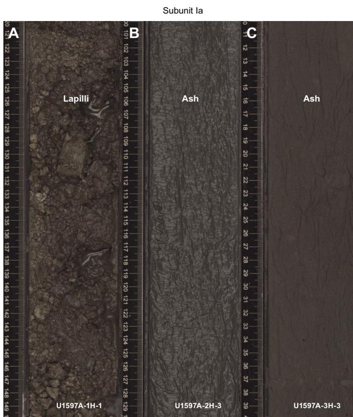
**Figure F7.** Dominant lithologies in Subunit Ia, Site U1597. A. Moderately to poorly sorted gray lapilli-ash observed in the uppermost core section. (B) Greenish dark and (C) very dark grayish brown ash intervals.
