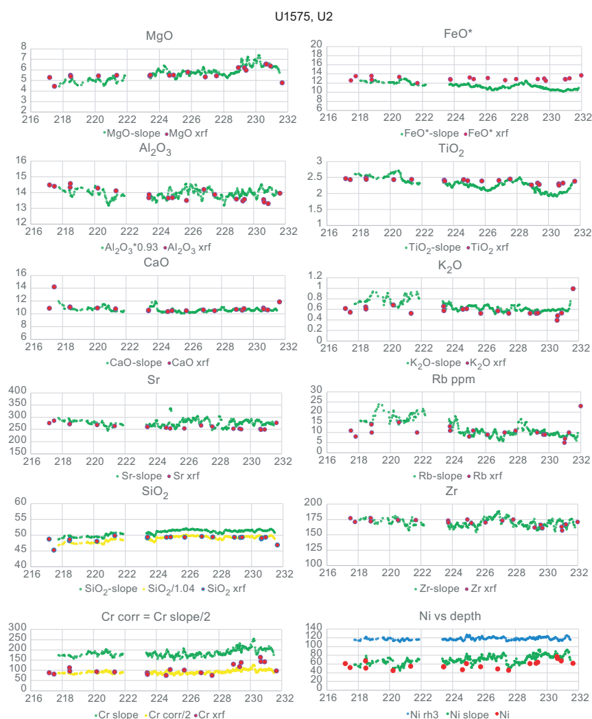
Figure F5. Comparison of slope-corrected concentrations to shore-based WDS XRF concentrations relative to depth (meters below seafloor), Hole U1575A Flow Unit 2.
