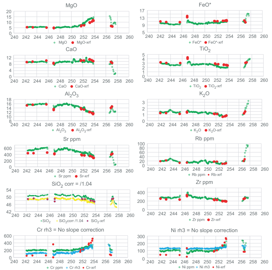
Figure F8. Comparison of slope-corrected concentrations to shore-based WDS XRF concentrations relative to depth (meters below seafloor), Hole U1578A Flow Unit 6.
