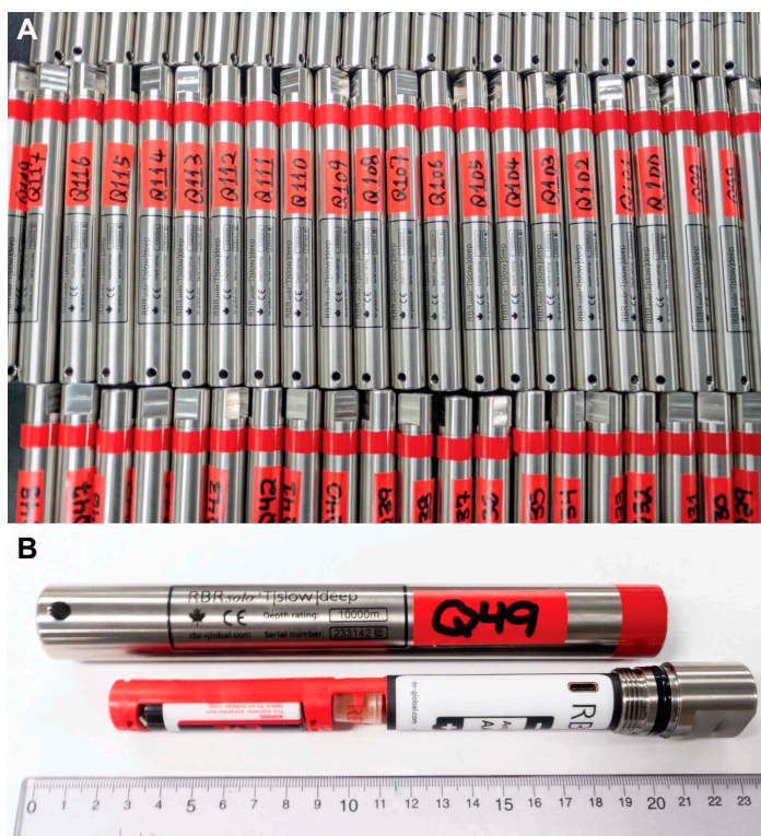
Figure F27. Temperature-sensing data loggers, Expedition 405. A. Temperature sensor instruments ready for attachment. B. An open RBR Solo 3 T instrument, revealing its internal components, including battery, silica desiccant, and USB-C port for programming and data retrieval.
