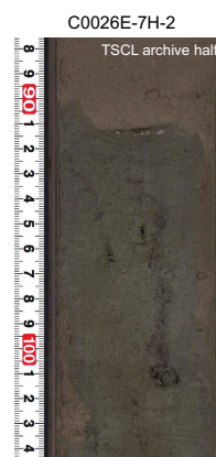
Figure F32. Drilling disturbance (flow-in) seen during piston coring, Hole C0026E.
